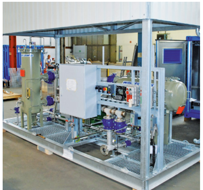
↑ Refueller loading skid
